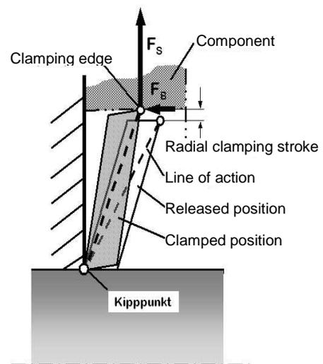
Fig. 5 Functional principle of the knee-lever effect
