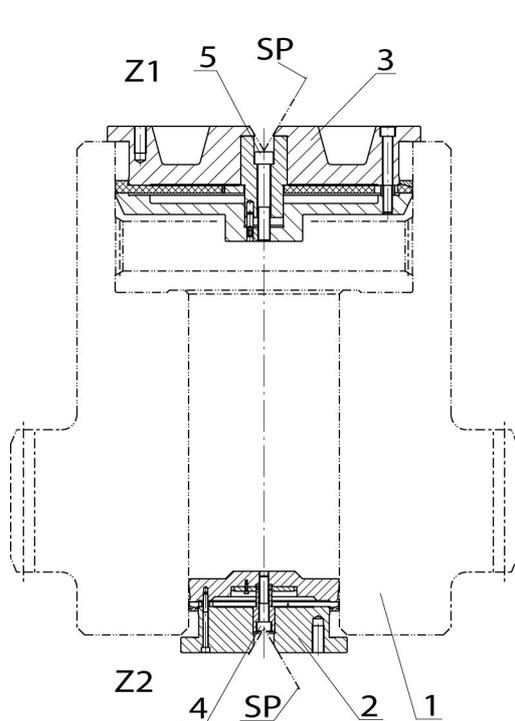
Fig. 16 Flat-mandrel clamping elements as centring inserts in a hollow shaft.
