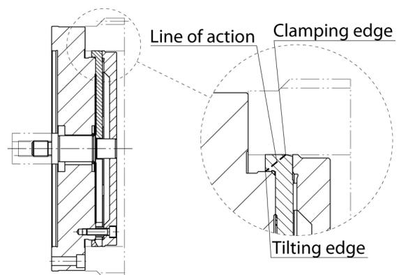
Fig. 8 Flat mandrel clamping element
