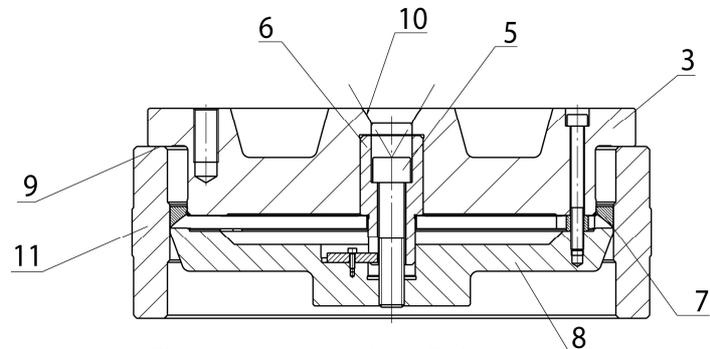
Fig. 17 Lower centring insert Z2 for a hollow shaft as shown in Fig. 16
