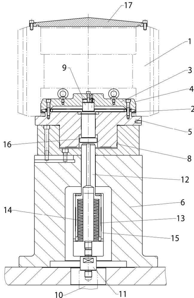
Fig. 20 Flat-mandrel clamping element with hydraulic expansion clamping chuck for milling of a large planetary pinion, power activated
