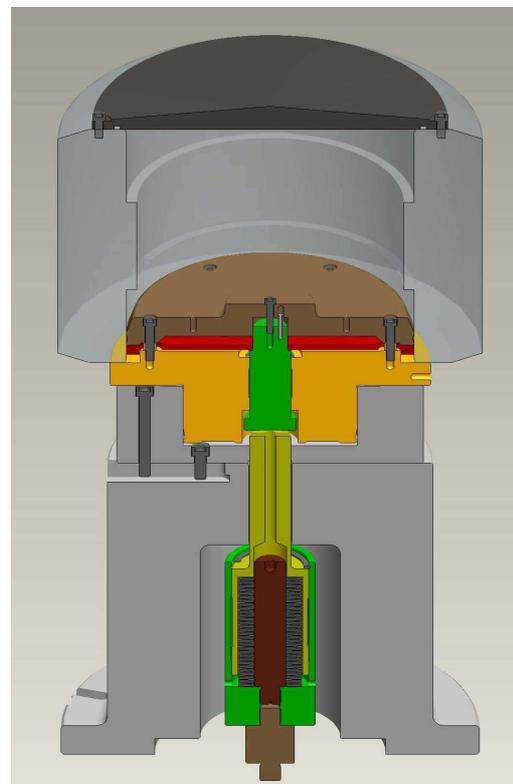
Fig. 21 Flat-mandrel clamping element with hydraulic clamping chuck for milling of a large planetary pinion, power actuated. 3-D view
